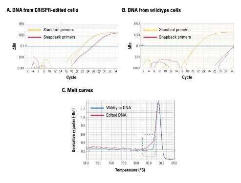
*Figure 2. The CRISPY assay specifically quantifies successful CRISPR/Cas9 editing events when performed on isolated genomic DNA. Amplification curves from (A) DNA isolated from CRISPR-edited cells and (B) DNA isolated from wildtype cells. (C) Melt curves from A and B.*
